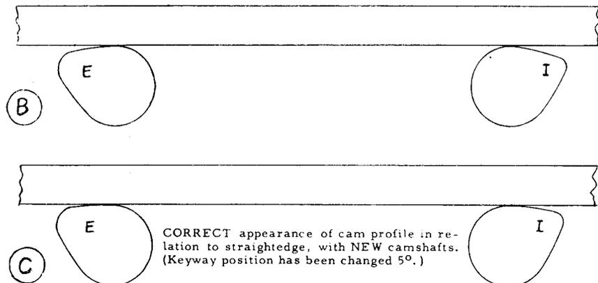
**Fig. GR6 — View B shows next to latest valve camshaft setup. Other view shows latest camshafts. Note relationship to straightedge.**
