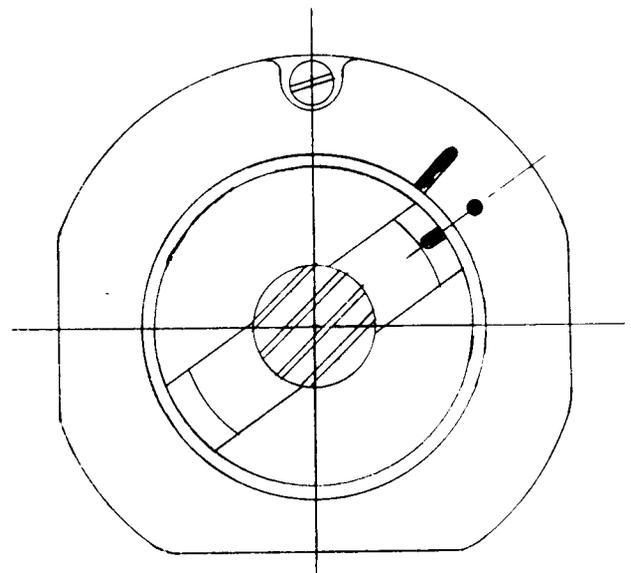
Fig. GR4—Magneto face plate showing double timing marks.
