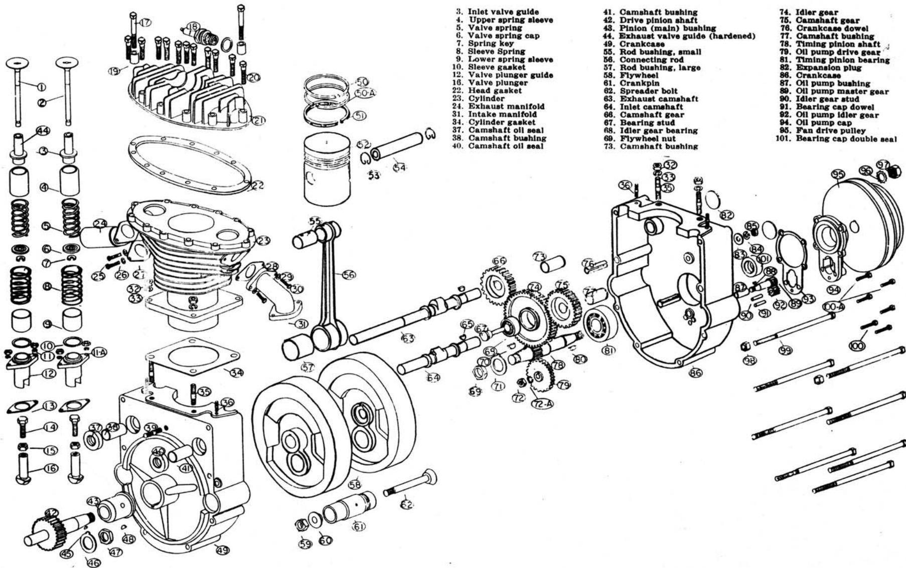
Fig. GR5—Exploded view of T head type engine used in Gravelly model L tractor. Note flywheels (58), pin (61), rod (56) and shafts (42) and (78) are actually components of a built-up type crankshaft assembly.
