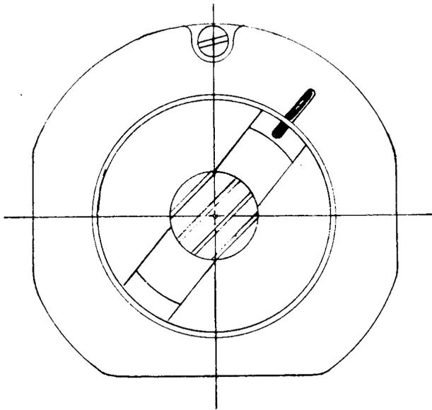
Fig. GR3—Magneto face plate showing one form of timing marks.
